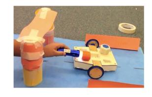
**Fig. 7** Child uses flashlight to trigger light sensor
