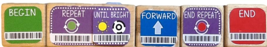
**Fig. 8** Programming blocks for Light Sensor Program. Using this type of program, children programmed their robots to continue forward along the map until a flashlight shines into the light sensor. Once the light is detected, the robot stops moving
