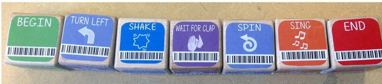
**Fig. 4** Sample program for the sound sensor
