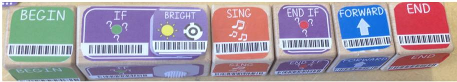
**Fig. 9** Conditional Statement Program. Children created conditional programs that allowed their robots to sing if it was “daytime” (i.e. the light sensor detects brightness) and “go home” (i.e. move forward) if it is “not daytime” (i.e. the light sensor does not detect brightness)
