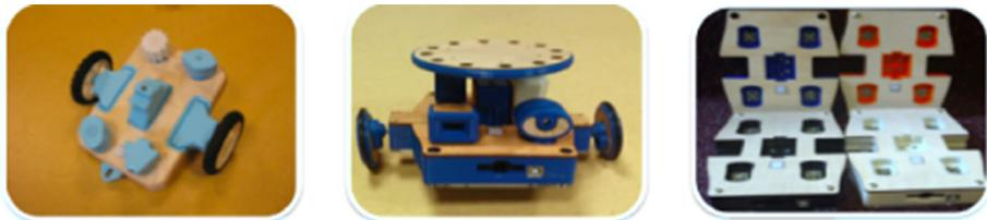
**Fig. 1** Design iterations of KIWI prototype. The design changes the KIWI prototype went through based on pilot testing with children and teachers. Changes include: adding design spaces for building and creating with crafts, creating a see-through bottom to examine the inner workings of KIWI, and making the robots more colorful
